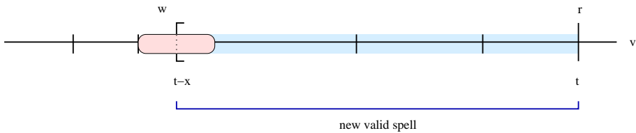
Fig. 1. Looking at boundary conditions for the maximum spell length constraint. A maximum spell length of x defines an interval [t - x, t) for the start of a spell ending at time t . A new spell can be formed if the RO at time t - x is added to the model.
